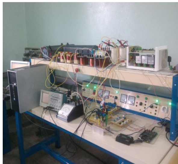
Fig.6. PWM Rectifier With the function of an Active Power Filter experimental test bench.
